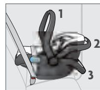
**NOTE:** The carry handle must be locked in any (3) positions when in use (p. 29).
