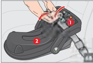
**STEP 6B:** Close the top section of the lock-off over the belt **1**. Second, close the bottom section of the lock-off over the belt **2**. Make sure you push the bottom of the lock-off all the way down until you hear an audible click.
