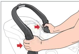
The carry handle must be locked in any three (3) positions when in use:
