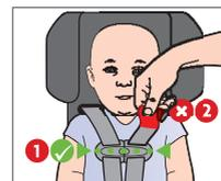
Retainer clip must be at armpit level **1** and harness straps should be snug **2**.
