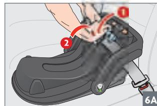
**NOTE:** Check that the base doesn't move more than 1 in side to side at the belt path. If movement is more than 1 in, twist the buckle and then fasten the seat belt to help secure fit.
