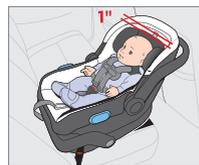
The top of the child's head should not be less than 1 in from the top of the headrest when in its highest position.
