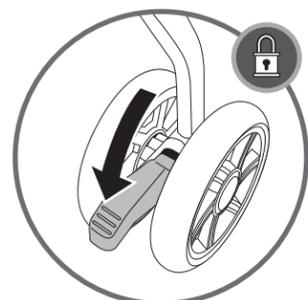
Press pedal down with foot to lock brake.
