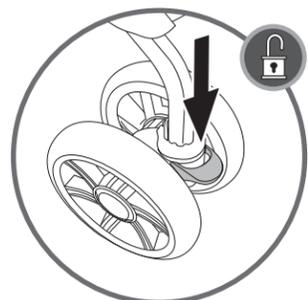
Press pedal down with foot to unlock swivel.
