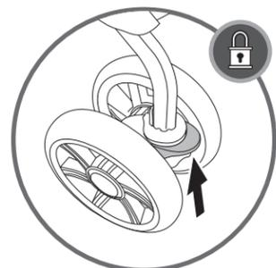
Press pedal up with foot to lock swivel.
